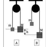
Now since the blocks are tied to the rope, they must be traveling at the same speed at all times (before M hits the ground). So if v is the speed of M at position B, then v must be the speed of m at position B. In other words, the gain in KE of the two blocks in going from A to B is:  $\Delta KE = \frac{1}{2} \text{ mv}^2 + \frac{1}{2} \text{ Mv}^2$ .
